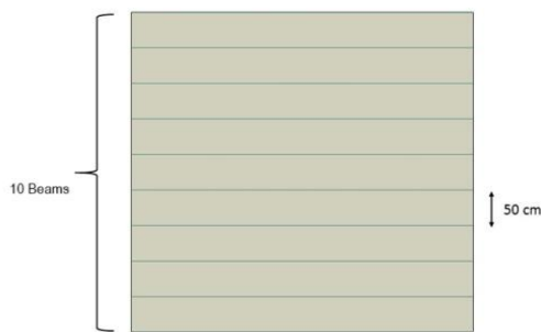
Figure 3. Arrangement of roof beams.
